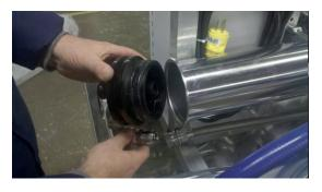
Remove the clamp at the end of the membrane housing (end where the clear hose come out). Use a ½" key.
