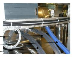
3b- Optional set up; If you only want to double the brix level and boil the concentrate right away, you can set the concentrate hose in another tank that will feed the evaporator.
