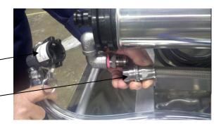
Remove the cap by pulling it out of the SS housing
