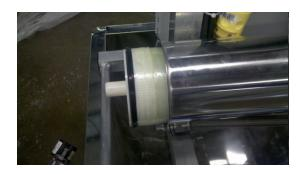
Push in the member with to U-cup last. IMPORTANT: It's very likely that a new membrane will come with the U-cup upside down. Remove it and make sure it's in the right position (see the next picture)
