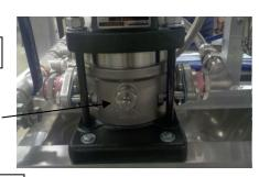
Remove the prefilter canister an remove the prefilter. Next time you run, change the prefilter or keep the old one where it won't freese between uses.
