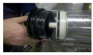
Insert back in the housing the black cap, making sure the pin of the membrane slides in the cap. Notice that it's possible that it will be quite hard to push the cover all the way in.
