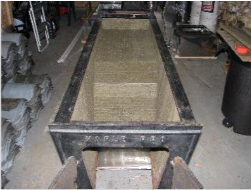
Insulating panels installed in the evaporator.
