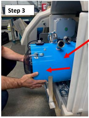
Remove the tank as shown.
